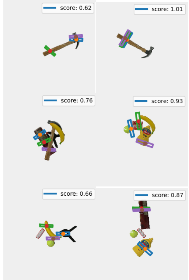
Fig. 2: Examples of what the model sees during grasping for scenarios isolated, pile, packed top to bottom, and GGCNN and GR-ConvNet, on the left and right respectively.
